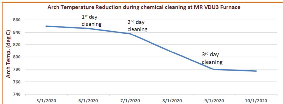
**Continuous reduction in Arch Temperature during chemical cleaning**
