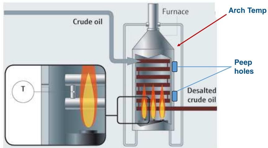
**Arch Temperature** of the furnace is measured at the junction of radiant section and convection section
